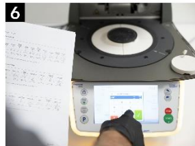
6 Enter firing parameters into the furnace (see NexxZr Glaze Spray Instructions for Use).
